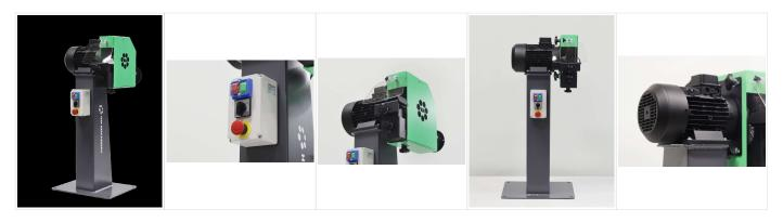
The HM model ZP 45 Tube deburrer can remove burrs from both the inside and outside of tubes in one operation, thereby reducing deburring work-time significantly.
