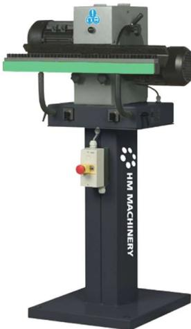
HM Sheet deburring machine model ZA 250 has a unique design, which ensures effective, safe and clean edge deburring of most ferrous and nonferrous materials utilising two abrasive flap wheels.
