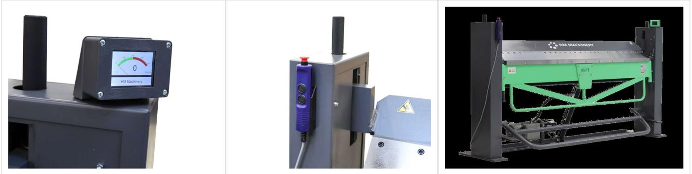
The HS-7SERGO, folder is actually a manual machine, which has been up-rated to offer a very efficient motorised option via a newly developed and patented, folding beam support cylinder system.
