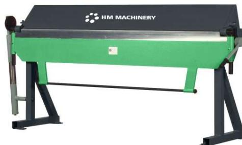
The MB 2000L folders are easy to operate, heavy, manual machines particularly suited for folding of the thin sheet metals.
