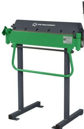
The MB Folder models MB 700L - 1300L are light, easy to operate, manual machines particularly suited for folding of the thin sheet metals.
